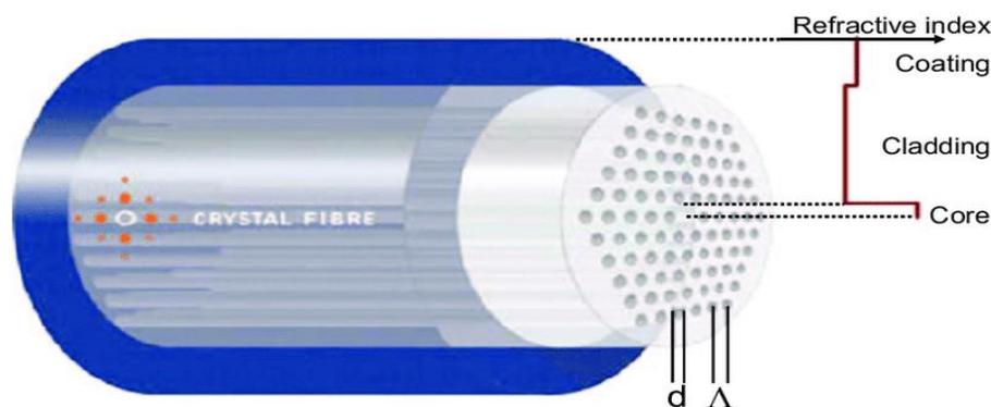
**Figure 1.** Solid core PCFs with microstructure cladding are the most prevalent design.
