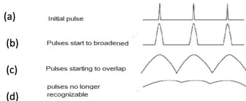
**Figure 2.** At various distances with time, the intensity of the pulses changes, (a) Original pulses, (b) pulses begin to broaden, (c) pulses begin to overlap, and (d) pulses become unintelligible
