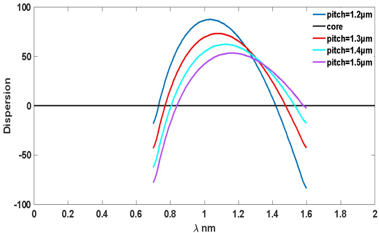
**Figure 6.** Variation of total TZDWs with  $\lambda$  for four different sets of  $\Lambda(1.2,1.3,1.4,1.5)\mu\text{m}$
