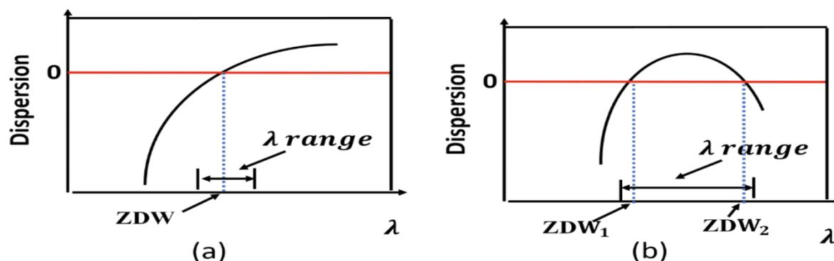
**Figure 3.** The wavelength selection range for (a) one ZDWs, (b) two ZDWs.
