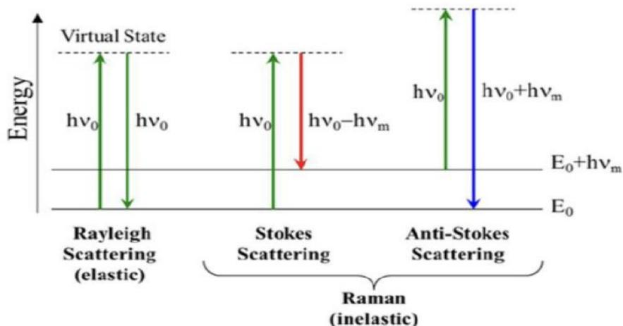
**Figure 4.** Diagram of Rayleigh and Raman Scattering quantum energy transitions
