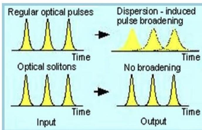
**Figure 5.** Waveform transformation of standard optical signals and optical soliton pulses throughout optical propagation
