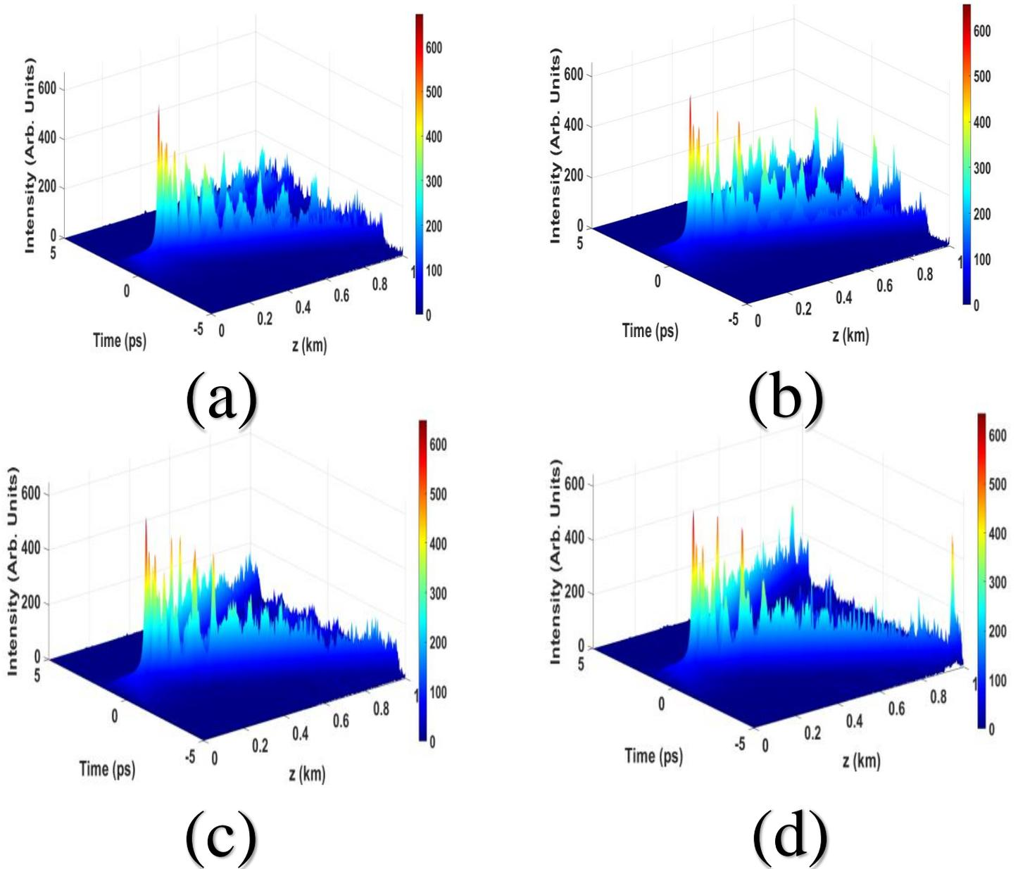
**Figure 7.** Temporal evolution of ultra-short higher-order ( $N = 3$ ) soliton propagation, when a-  $\Lambda = 1.2\mu\text{m}$ , b-  $\Lambda = 1.3\mu\text{m}$ , c-  $\Lambda = 1.4\mu\text{m}$ , d-  $\Lambda = 1.5\mu\text{m}$
