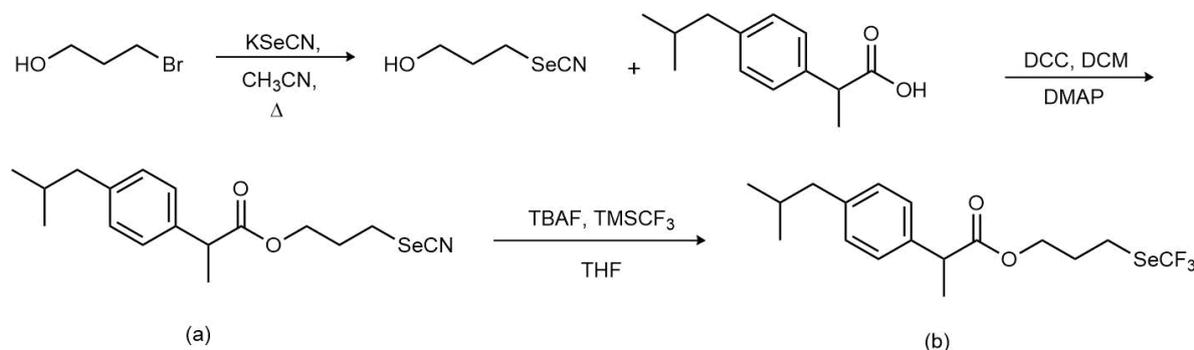
**Scheme 9.** Synthesis of organoselenides-ibuprofen derivatives. Compound (a) cyano substituted and compound (b) trifluoromethyl substituted
