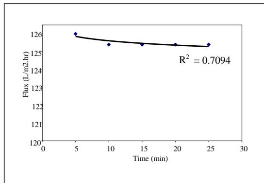
**Figure 1** Flux versus time for 100 kDa PES membrane
