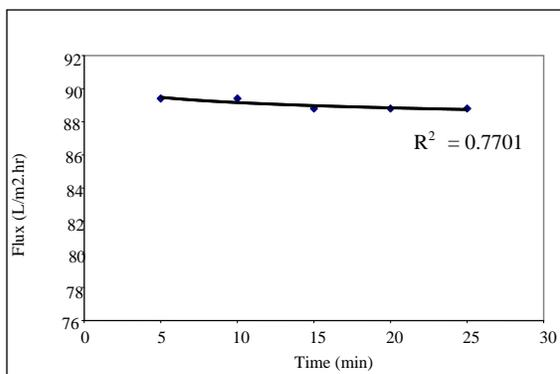
Figure 3 Flux versus time for 10 kDa PES membrane
