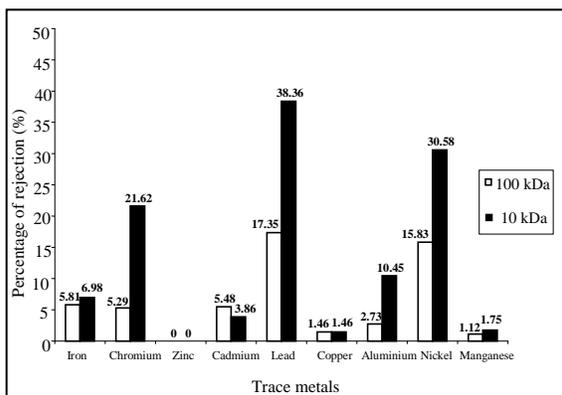
Figure 7 Comparison of trace metal’s rejection performance between 100 kDa and 10 kDa PES membranes
