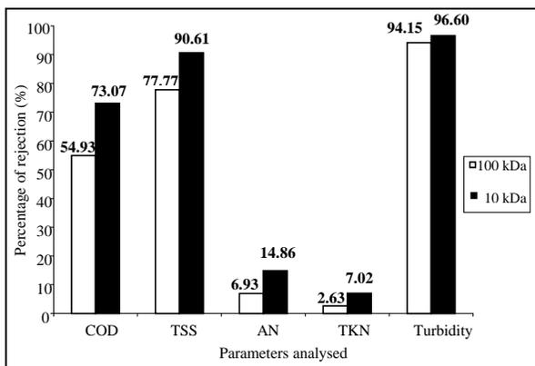
Figure 6 Comparison of selected parameter’s rejection performance between 100 kDa and 10 kDa PES membrane
