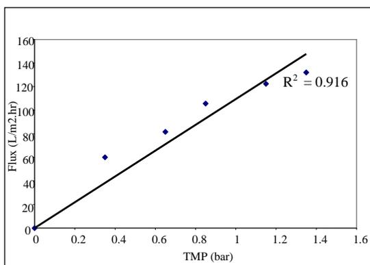
Figure 4 Flux versus TMP for 10 kDa PES membrane
