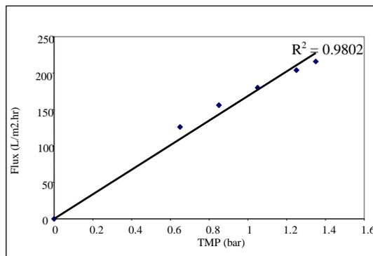
**Figure 2** Flux versus TMP for 100 kDa PES membrane
