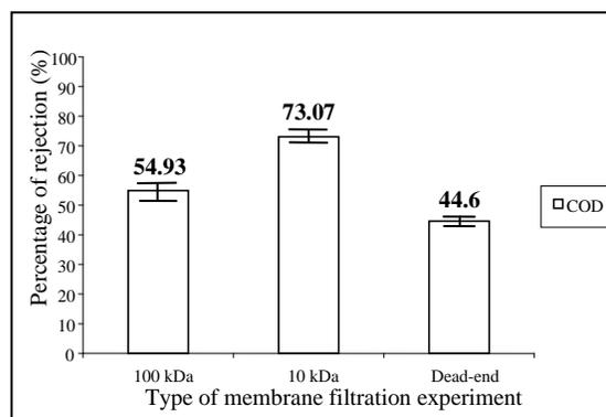
Figure 5 Comparison of COD's rejection performance between cross-flow and dead-end filtration
