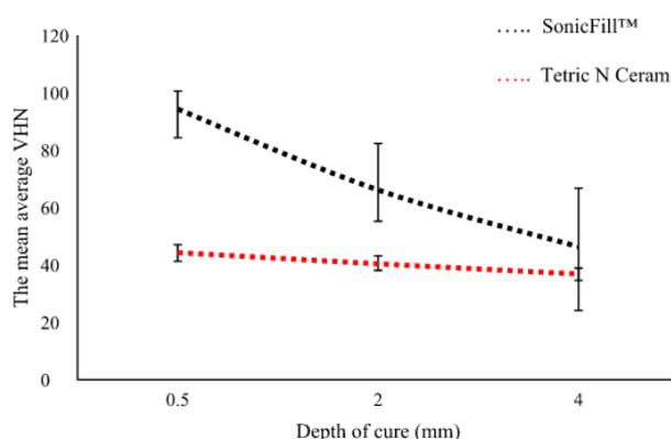
Figure 3: The mean average hardness in increasing curing depths
